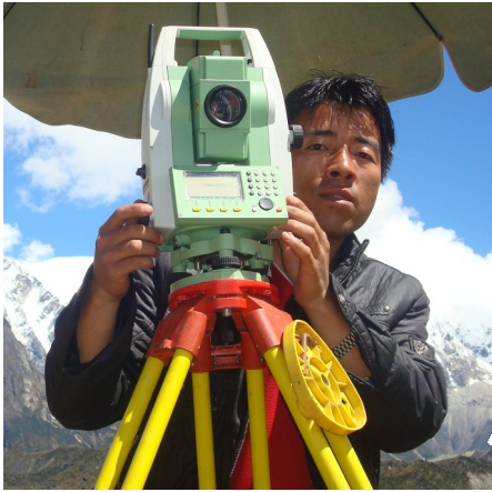
A survey engineer observes with a Total station
