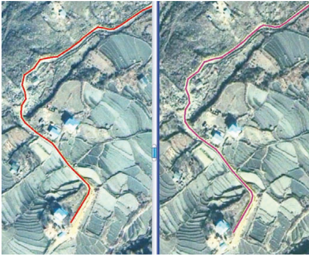
Figure 4, Monoplotted track in one Ikonos image (left) backprojected into second image (right) to illustrate high metric accuracy.
