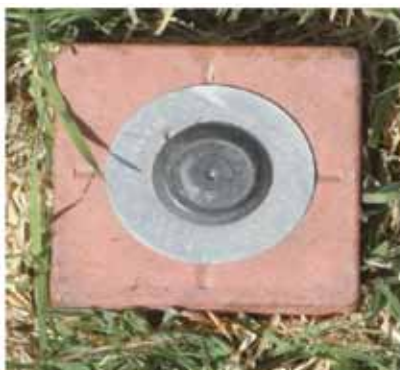
Feno peg control point
